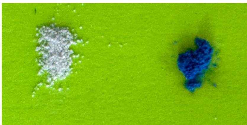
Figure 15 - Product resulting from the experiment, pure MOF-5 and with adsorbed methylene blue (MB)
